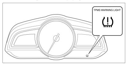
The TPMS system may have been improperly initialized when the initialization was performed on certain types of rough road surfaces. Then, when driven on smooth road surfaces, the TPMS system may detect improper tire air pressure. The DSC HU/CM control logic has been changed for this concern.
