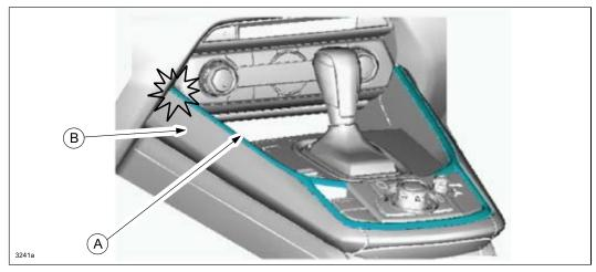
The noise may be caused by the chrome decoration panel (A) interfering with the side panel (B). To eliminate the noise, a noise prevention tape has been added to the front console.
