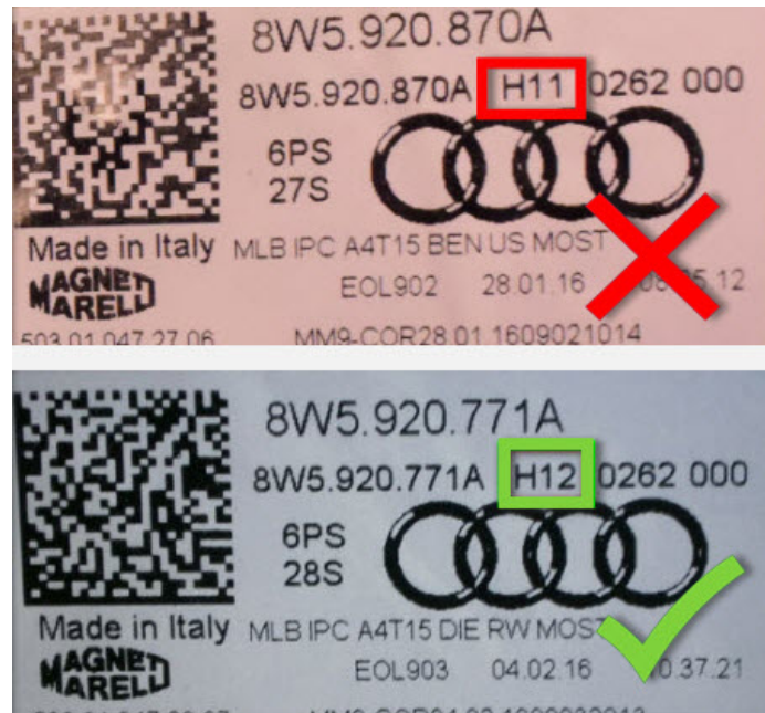
Figure 2. Hardware level below H12 (top) must be replaced. Hardware level H12 (bottom) does not need to be replaced.
