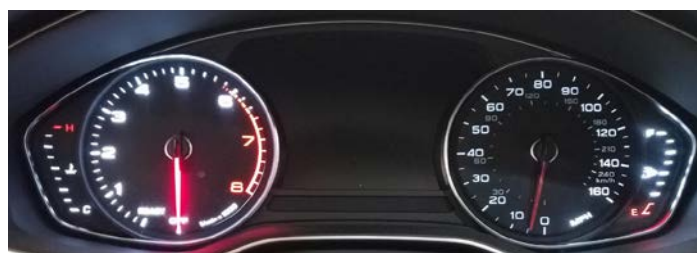
Figure 1. Example of inoperative driver information display with inoperative backlighting.
