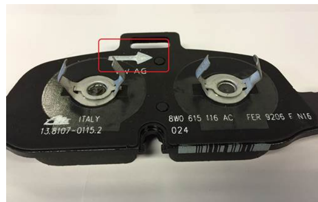
Figure 4. Arrow showing correct installation direction.
