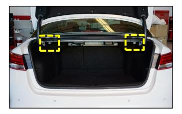
2. Pull the release cable towards the rear and rotate the handle left or right while applying moderate twisting force.
