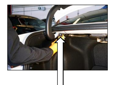
3. If the handle stays intact, no further action is required. If either of the release cable handles break during inspection, proceed to the Service Procedure on Pg. 3.
