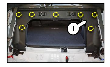
9. Remove four (4) bolts (J) securing the seat latch release, as shown.
