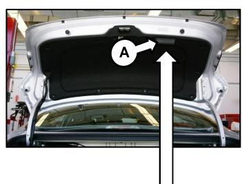
2. Remove two (2) screws (B) from the trunk grab handle.
