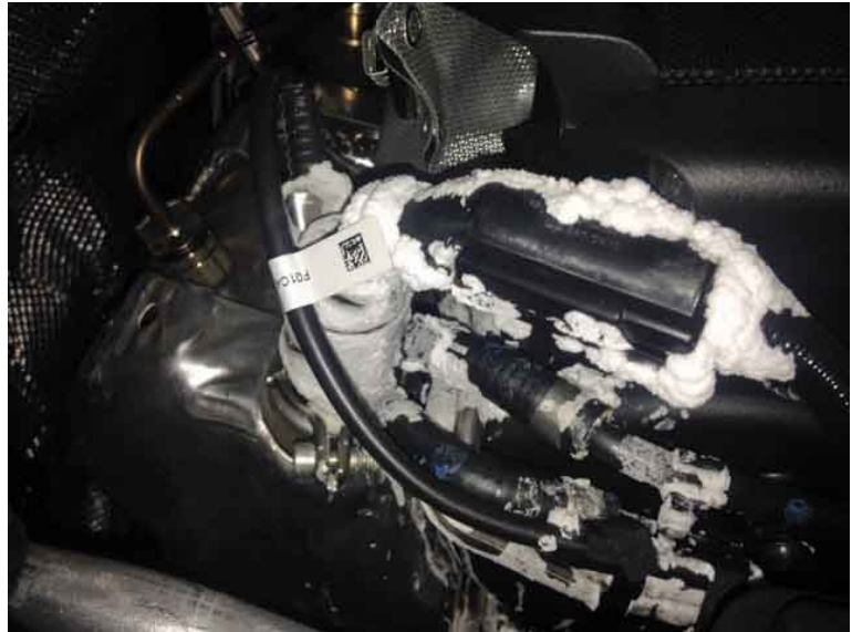
Figure 1. Evidence of leak –AdBlue residue.
