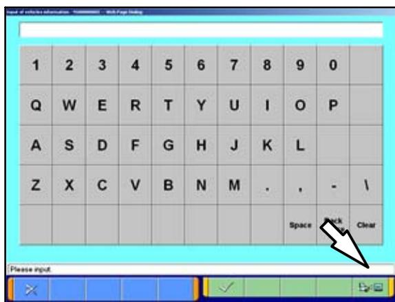
7. Click on the icon in the lower RH corner of the screen to have MUT-III automatically read the VIN. If a message appears advising the VIN cannot be input automatically, enter the 17 digit VIN.
