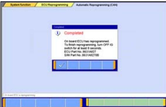
21. Once the programming is completed, the **Completed** dialog box is displayed.
