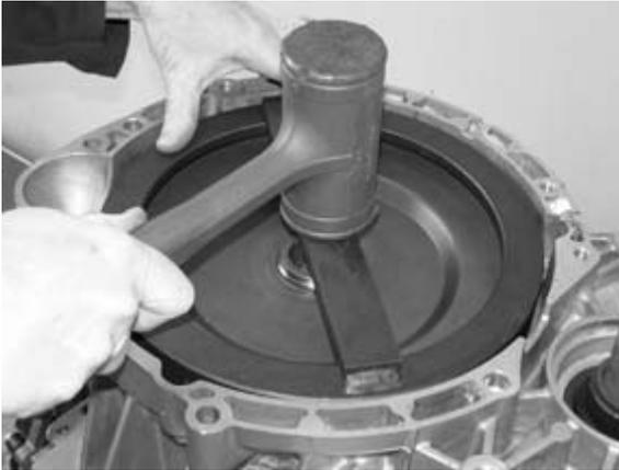
g. Use special tool cover installer (MB998323-01) with a dead blow mallet to seat the cover into place.
