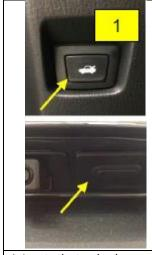
1. Locate the trunk release and engage the trunk release button
