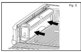
Push bin assembly tight to side of wall of truck box and align fastener holes with M8 and M6 rivnuts. Ensure fixed tie down loops slide through assembly cutouts. (Figures 5 and 6).
