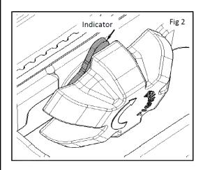
2) Make sure indicator is in the unlocked position. See Fig. 2  $\,$
