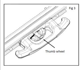
Position cleat into channel until flush with channel opening. Rotate thumb wheel clock-wise until tight (22 in lbs max.)See Fig. 3
