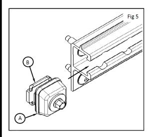
5) Slide endstop into channel opening. Channel to be positioned between body (A) and plate (B). See Fig. 5
