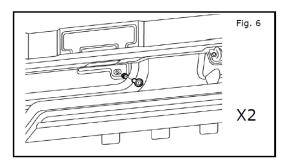
Open bin assembly lid and install M8 spacer and M8X33 bolt. Install in (2) locations (Figure 7). Tighten screws to 10Nm.
