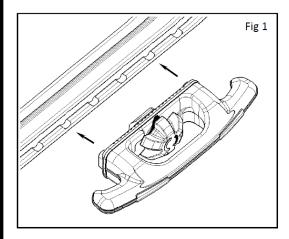
Line up lugs on underside of cleat with notches in the channel. See Fig. 1
