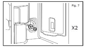
7) At front and rear tie down holes, install M6 x 25 shldr bolt and washer (2) locations. Tighten bolts to 5Nm.
