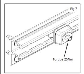
7) Torque bolt to 25Nm using 10mm socket wrench. See Fig. 6
