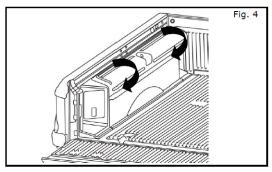
Position bin assembly near sidewall of truck box (Figure 4). Angle top of bin assembly so upper tabs are positioned behind Utili-trac trail.
