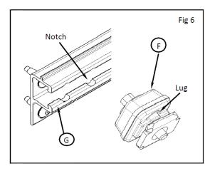
6) Align lugs on body (F) to notches on channel (G) in desired location. See Fig. 6
