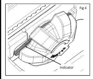
4) Indicator should be in locked position as shown. See fig. 4
