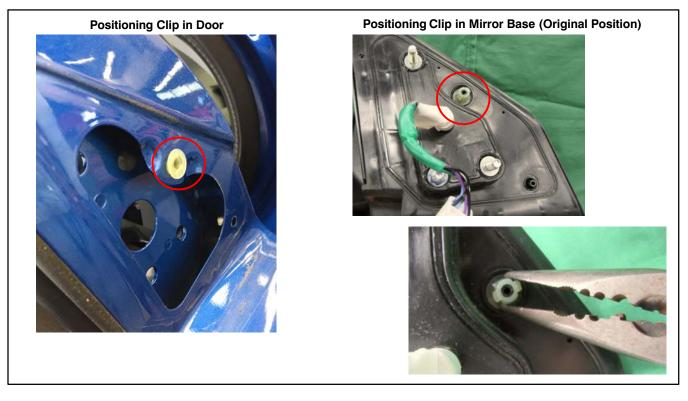
Reinstall the door mirror assembly onto the door panel.
