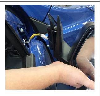
2. Once the door mirror is removed, locate the positioning clip.
