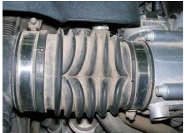
Figure 2. Vacuum in the air duct hose between air filter and throttle valve.
