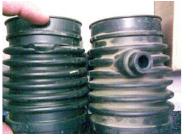
Figure 3. Crack in the intake hose.
