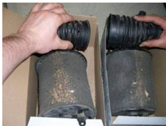
Figure 1. Example of excessive dirt on air filters.
