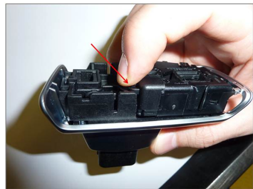
Figure 2. Apply force to fully install the cover.
