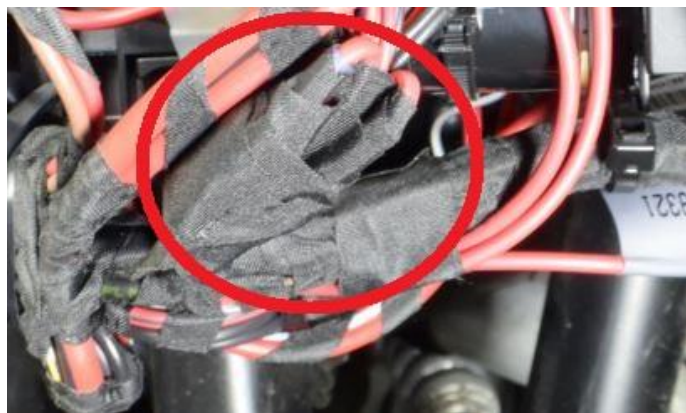
Figure 31. Original power wires that have been folded back into the harness and taped.
