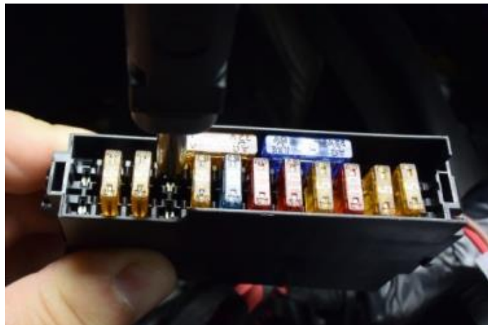
Figure 15. SB4 battery power feed wire terminal.
