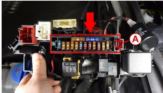
Figure 10. Fuse block ST1 with tab for removal (A).
