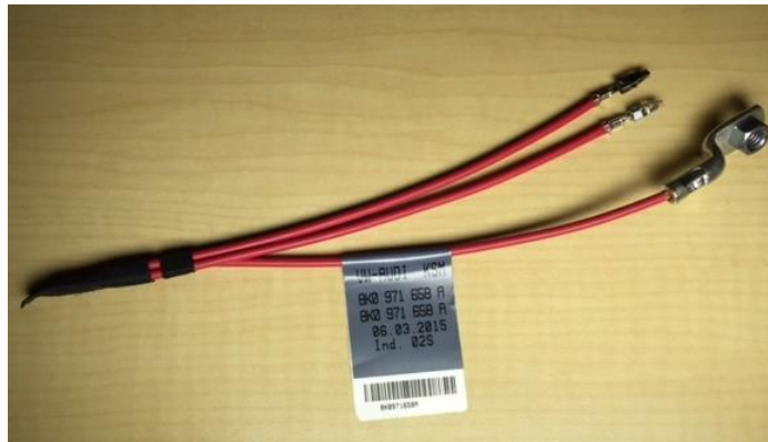
Figure 23. New battery power feed wiring.
