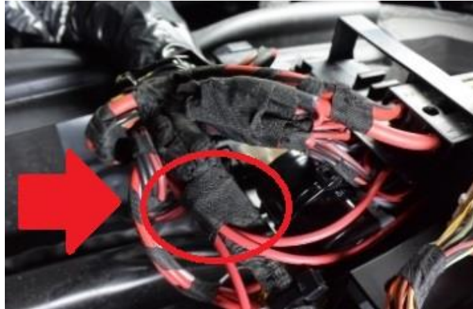
Figure 32. Repair harness secured.
