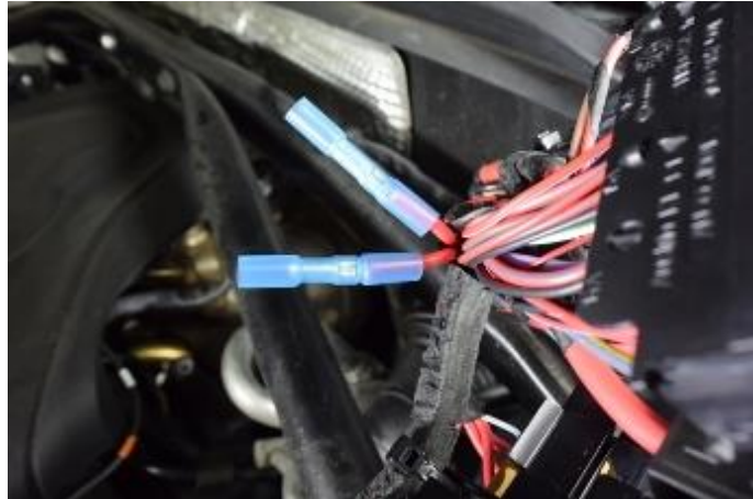
Figure 20. Installed crimped butt connectors.
