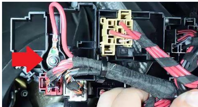
Figure 27. 10mm nut to be removed from the bottom of fuse panel B -SB-.
