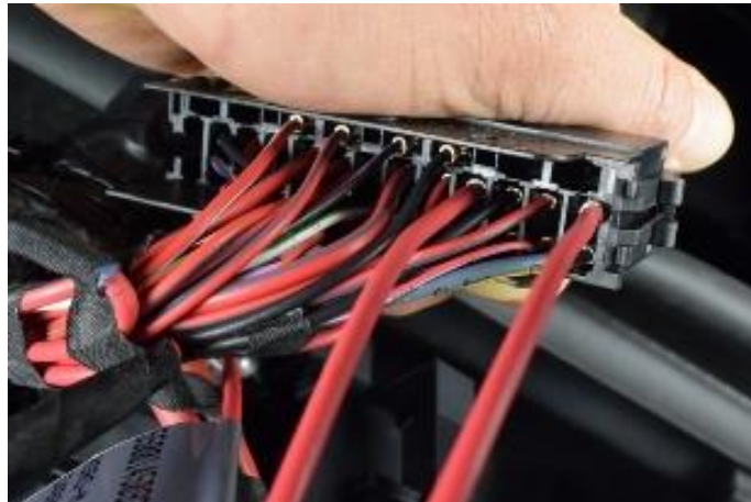
Figure 24. New battery power feed wiring installed into fuse block.
