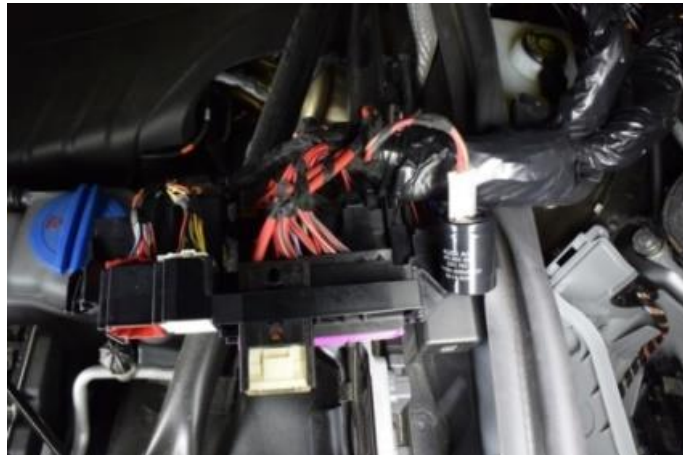
Figure 8. Suppression condenser removed from fuse panel B -SB-.
