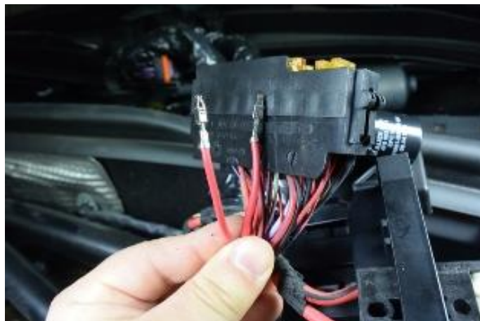
Figure 17. Both power feed wires removed.
