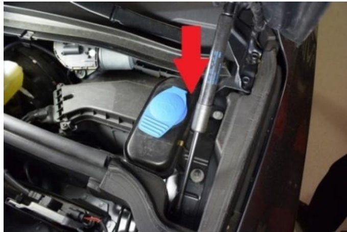
Figure 3. Washer fluid filler reservoir filler tube.
