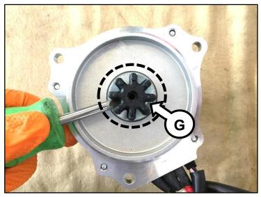
8. Install the new improved flexible coupling onto the steering column.
