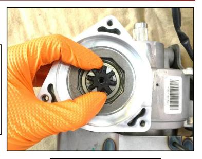
Reassemble all other components, confirm MDPS operation and test all multi function switch functions for proper operation.
