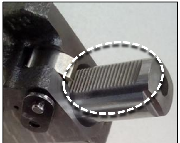
New tensioner design with finer pitch on teeth (1.5mm)
