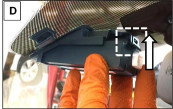
After reattaching the camera, perform the LDWS calibration using SST 09890 3V100 by referring to the "Body Electrical System → Lane Departure Warning System (LDWS) → Repair Procedures" chapter in the applicable Workshop Manual on KGIS.
