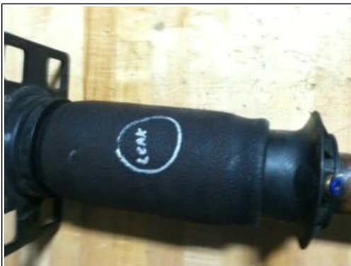
Figure 4 example of marking where air leak was found
