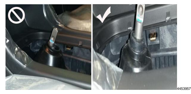
5. Ensure the transmission control lever boot is secured as shown above.
