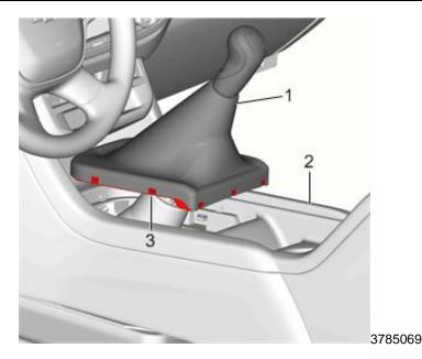
9. Position the boot tabs flat on the console opening and push downward on all four sides of the boot (1) in order to engage the boot retainers (3) with the floor console (2).
