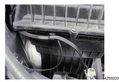
10. Install the edge clip (13596781) on the third lower rib of the air cleaner assembly and loosely secure the coolant heater cord.
