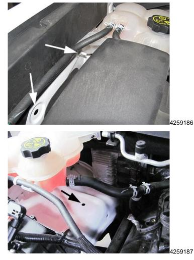
5. Locate the 2 mounting holes and 1 stud to attach the tie straps as shown.
