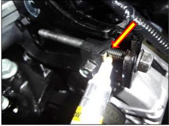
3. Loosen the top alternator mounting bolt.
