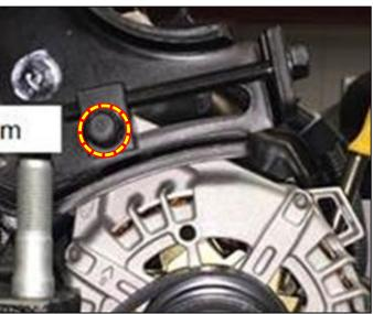
7. Replace with a new bolt. Do not tighten fully.
