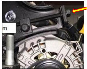
6. Remove the top alternator mounting bolt.
