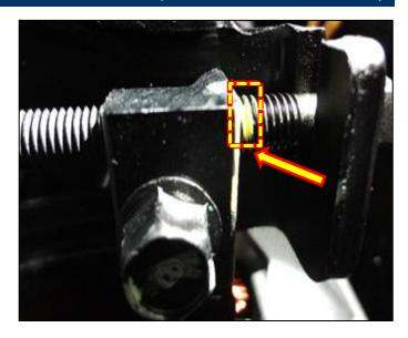
9. Verify the belt has the proper tension and adjust it if needed.
