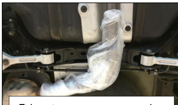
Exhaust near rear cross member
