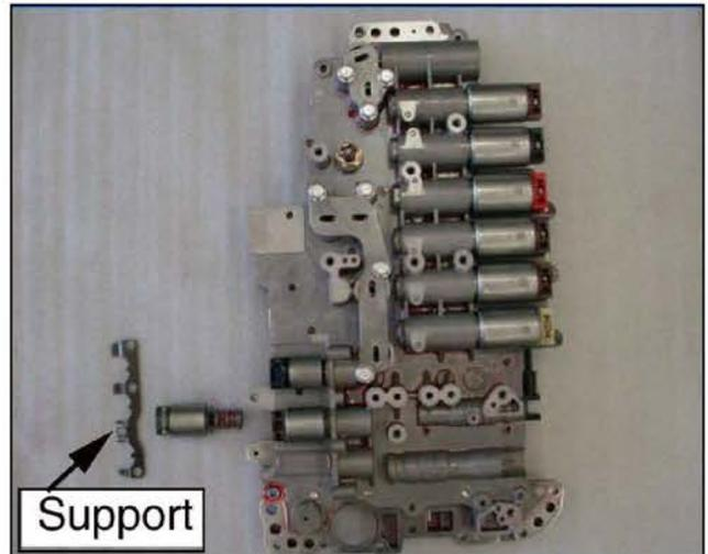
14. Install a new E-module and torque to specification.
