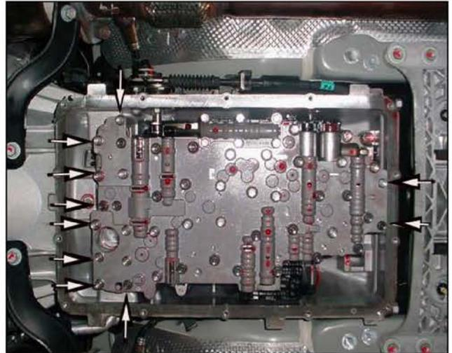
8. Remove 8 bolts and remove the E-module.
