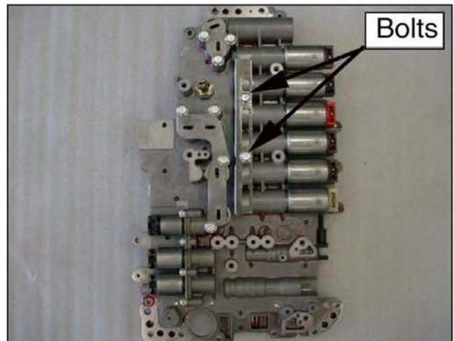
12. Use a magnet to remove the pin and remove the related solenoid. Install a new solenoid. Reinstall the pin and the solenoid support.
