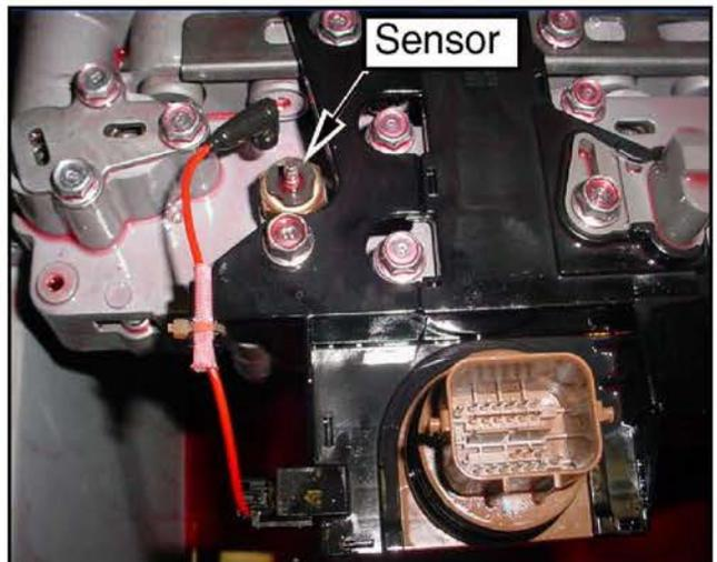
10. Refer to the solenoid DTC recorded in Step 1 and replace the related solenoid. Refer to the PNC in the parts catalog.
