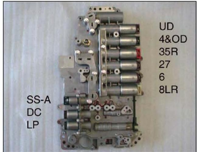
11. For UD, 4&OD, 35R, 27, 6 and 8LR solenoids: Remove two bolts and remove the solenoid support.
