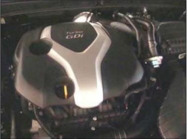
4. Remove the (1) 10mm O2 sensor connector bracket bolt from the cylinder head and move the bracket slightly away from the exhaust manifold.
