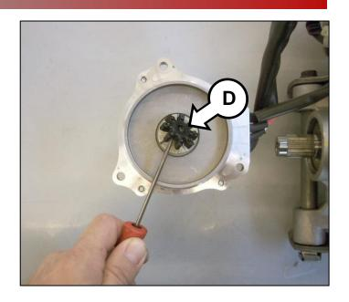
5. Install the new flexible coupling (E) onto the MDPS motor, as shown.
