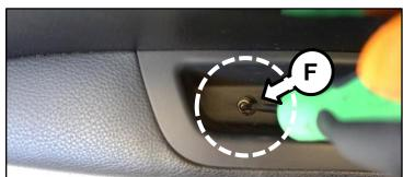
7. Remove the door panel. Leave the 2 master switch harnesses connected to allow for glass retaining bolt alignment in step 9.
