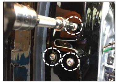
18. Remove the door module from the door without disconnecting the harness.
