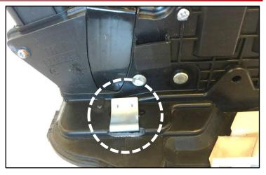
23. Apply silicone RTV sealant around the clip slot (R).
