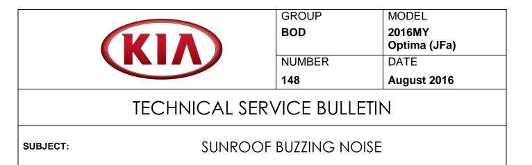
This bulletin provides information on some 2016MY Optima (JFa) vehicles, produced from September 28, 2015 to June 20, 2016, which may exhibit a buzzing noise that may increase with intensity in conjunction with the HVAC fan speed. This concern is caused by a loose sunroof weather strip vibration due to air leakage past the sunroof seal. To correct this concern, follow the procedure outlined in this bulletin to apply adhesive to the weather strip base.
