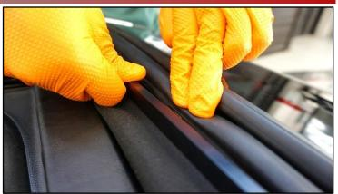
6. After ensuring that the adhesive has cured, open and close the sunroof several times to confirm proper installation of the weather strip.
