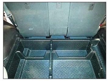
Remove the luggage floor covering panel and fuel pump service cover assembly (A).
