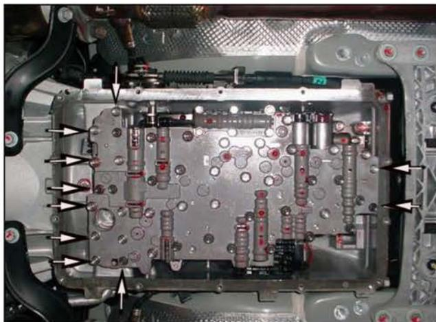
8. Remove 8 bolts that secure the E-module and remove the E-module.
