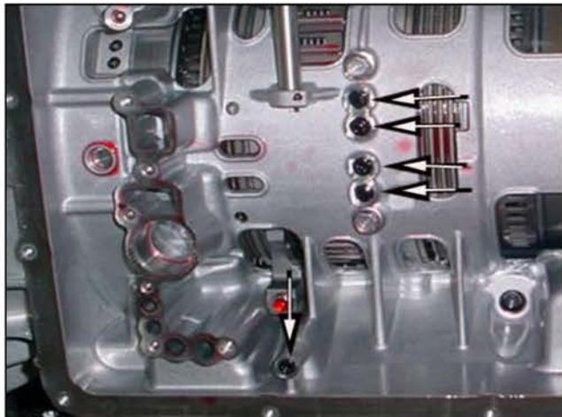
10. Carefully align the manual valve to the shift lever and reinstall the valve body.
