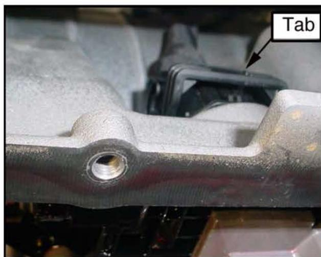
6. Use an 8mm or 5/16" hex socket to remove the drain plug and drain the ATF. Reinstall the drain plug.
