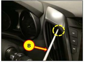
5. Securely position the puller tool to the upper left corner of the **RH Center Vent** and release the clips with a firm pull.
