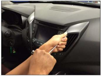
Use one hand to stabilize the hook end of the tool against the recessed portion of the center vent inner lip while pulling. This will help prevent slipping and scratching the center fascia panel near the vent. Firmly tug the T-handle of the tool to release clips.
