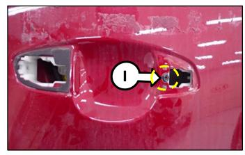
11. Loosen the three rear door latch attachment screws (J).
