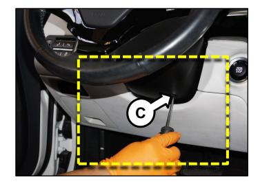
Use a plastic panel remover to separate the upper steering column shroud (D) from the lower section, as shown.
