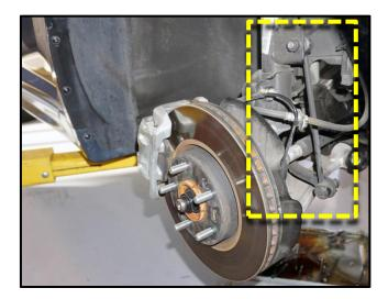
2. Install the improved front stabilizer links by reversing the removal steps.
