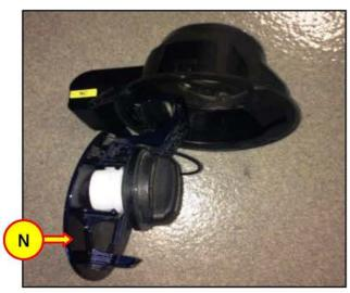
12. Install the removed fuel filler door (N) to the new housing (O).
