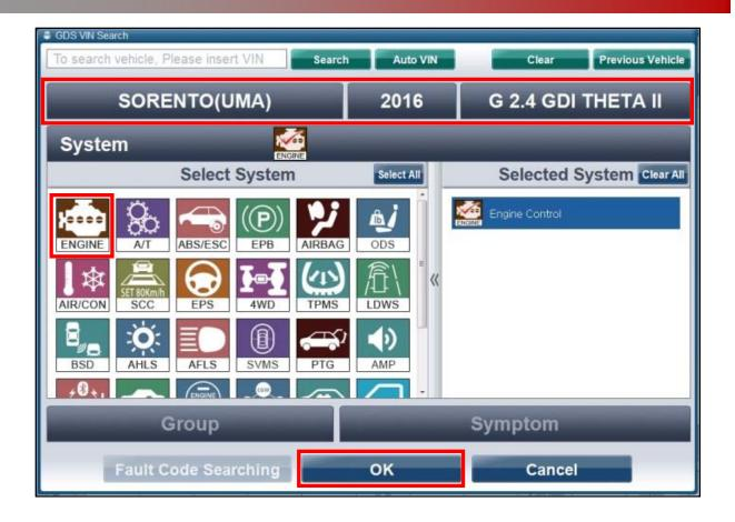
Select ECU Upgrade from the bottom right-hand corner. Next select Auto Mode, and then Engine. Perform event #289(JFa) / #290(UMa) in accordance with normal GDS upgrade procedures.
