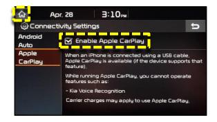
6. Connect the iPhone into the USB port using the Apple cable provided with the phone NOTE: Avoid using aftermarket cables.
