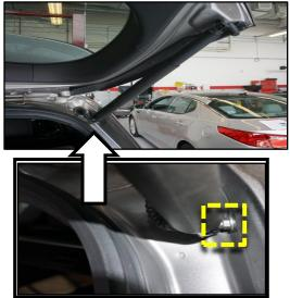
Using an open-ended 12mm wrench, verify the ball stud is securely attached to the body. If the ball stud is loose, tighten approximately ¼ of a turn, or until snug to the body.
