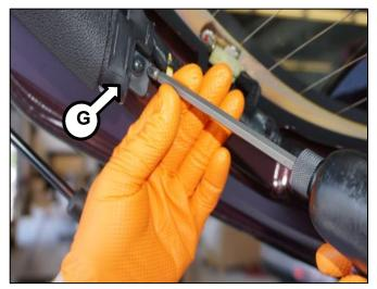
7. Dislodge the bottom portion of the tail gate trim (H) using a nonmarring trim panel removal tool.
