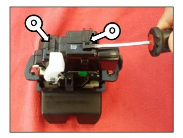
12. Remove gears (Q) and (P), from the cover by removing long and short pins. Discard the originally installed gear (Q), return spring below the gear (Q), and the latch cover, as they will be replaced later in this procedure.
