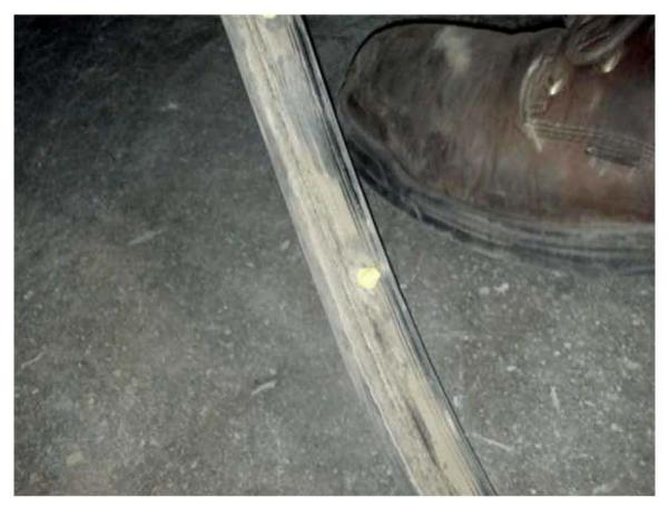
**Note:** A vehicle will sometimes show evidence of dirt/dust being pulled past the backside of the rocker moldings as shown above. A double sided tape is added to the moldings to help eliminate this condition.
