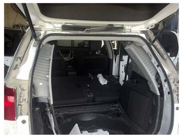
The cause of this condition may be that the dust/debris is working past the side door or liftgate sealing surfaces.
