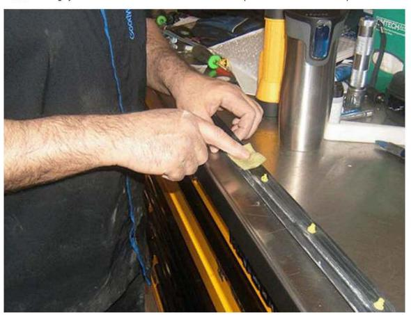
2.3. Apply 3M<sup>™</sup> Automotive Adhesion Promoter, or equivalent, to the entire length of the seals and between each push pin. The promoter should be centered in line with the push pins and cover an approximate area 15 mm (0.590 in) wide.
