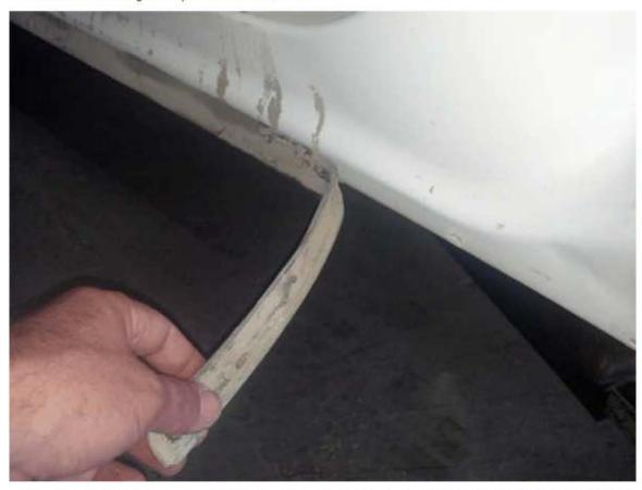
2.1. Remove the left and right rocker panel moldings (seals). Refer to Rocker Panel Molding Replacement in SI. Inspect the seals for any deformations or damage and replace as appropriate.
