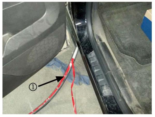
Note: The recommended size of the two-sided tape is approximately 1.5 mm (0.060 in) thick and 13 mm (0.500 in) wide.
