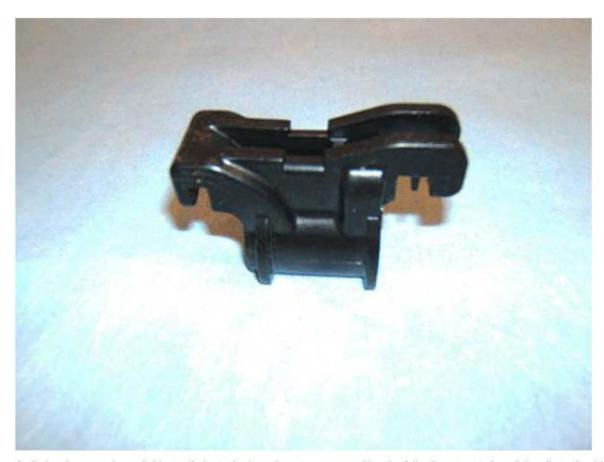
A clip has been made available to eliminate the lateral seat movement. Use the following steps to install the clip to the driver side seat. If the vehicle is equipped with a 6-way adjustable passenger seat, repeat the procedure on the passenger seat.
