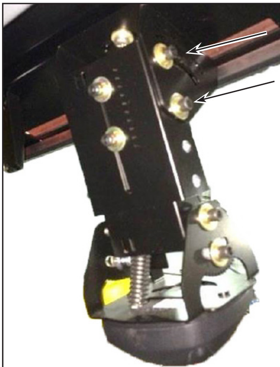
Figure 2 - Remove Four Bolts, Two Per Side
