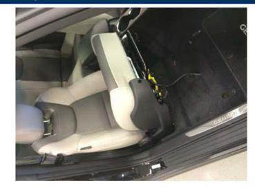
Locate the PODS unit under the seat.
