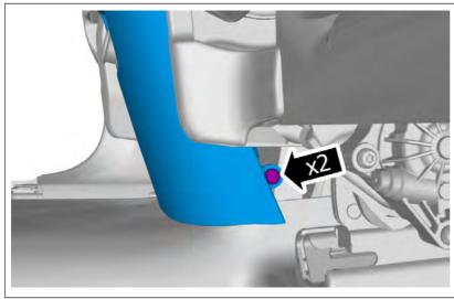
Remove the screw. On both sides.
