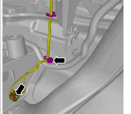
Loosen the clip. Remove the nut.
