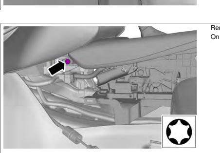
Remove the screw. On both sides.
