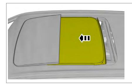
Lift the marked component forward.
