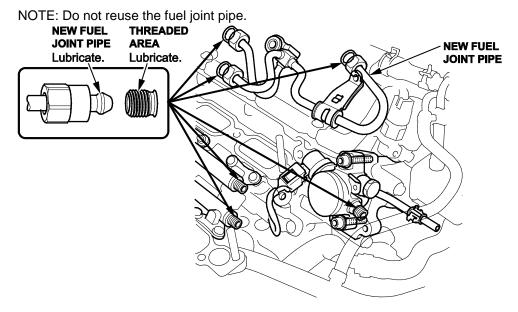
20. Tighten the fuel joint pipe nuts by hand until the end of the joint pipe is seated on the fuel rails and high pressure fuel pump.
