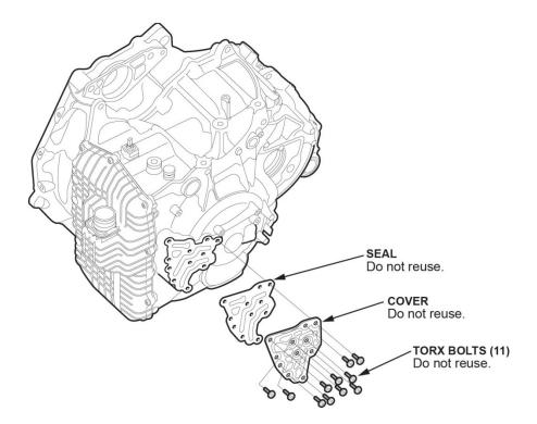
4. Replace the cover, the sealing gasket, and bolts with the new ones from the kit. Torque the bolts to **10.0 N-m (7 lb-ft)** in the sequence shown.
