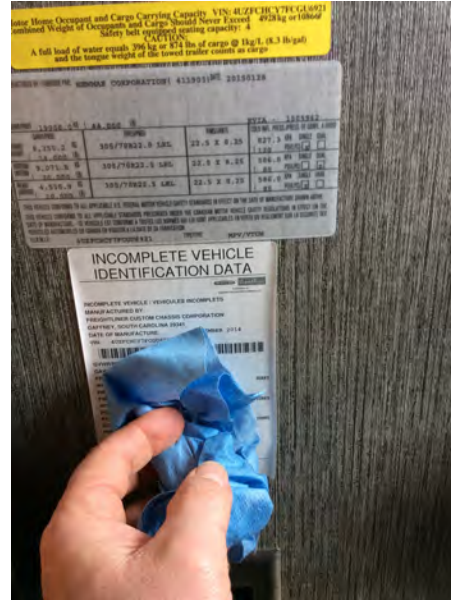
Method #1: Removing the Original Label
