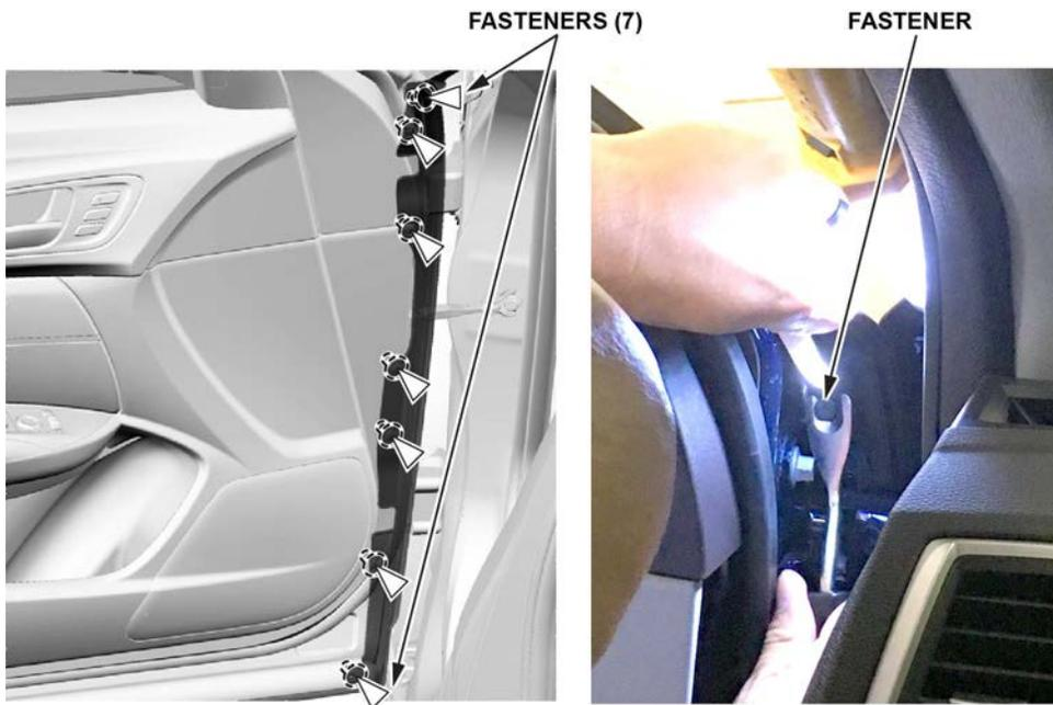
3. Once all the fasteners are removed, pull the seal up and out to remove it from the doorjamb area.
