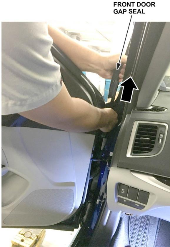
4. Install a new front door gap seal behind the door hinges, and install each fastener into its slotted hole.
