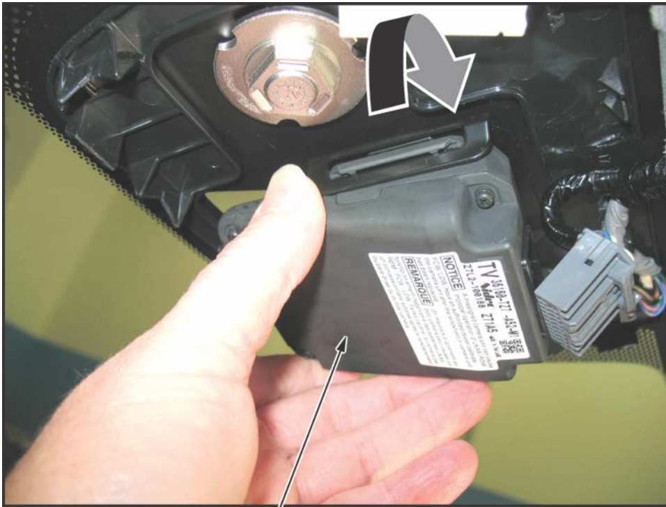
FRONT MULTIPURPOSE CAMERA UNIT
