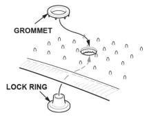
11. Use the special tools and a hammer to flare the lock ring.
